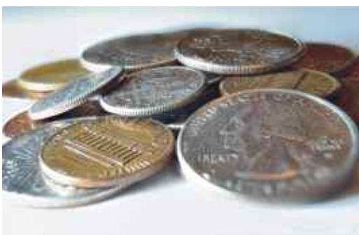
US penny uses 98% zinc coated with copper
